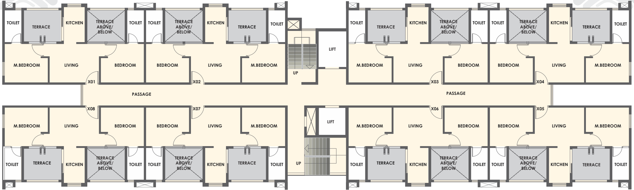
TYPICAL ODD FLOOR PLAN - BUILDING A1 TO A4 (1ST, 3RD, 5TH, 7TH, 9TH & 11TH FLOORS)
